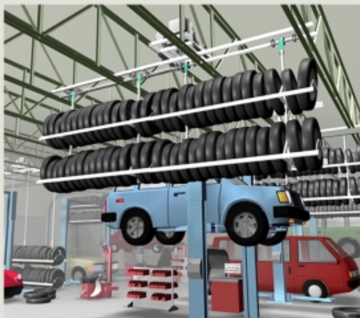
Overhead Storage with Versa Lift for Tires
